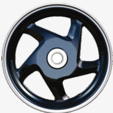
Wheel Rim Size : 12 inch Specifications : 2.15 x 12 inch PCD : 3 - Ø 80
